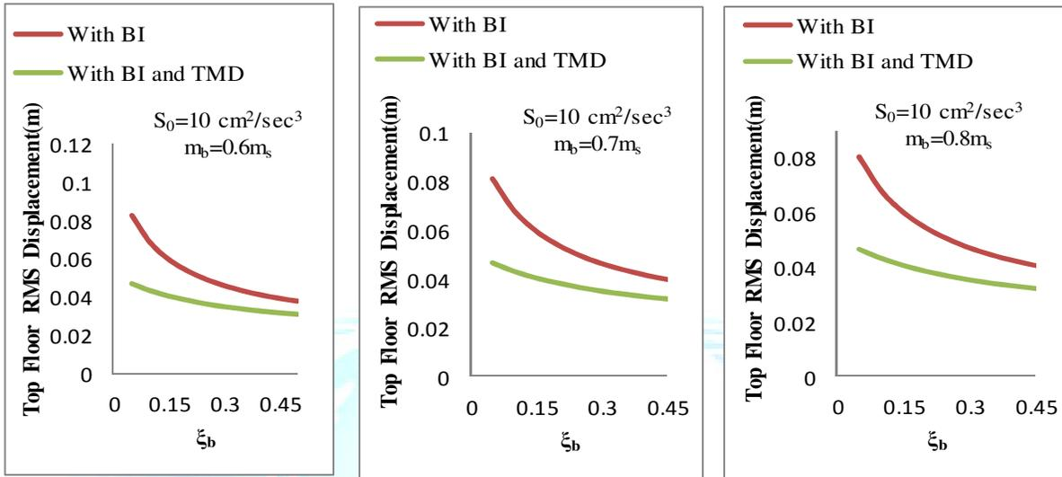
Fig.9 Variation of RMS displacement of top floor with damping ratio of base isolator,  $\xi_b$  for different mass ratio of base isolator and 5% damping ratio of structure,  $\xi_s$  and earthquake load,  $S_0 = 10 \text{ cm}^2 / \text{sec}^3$
