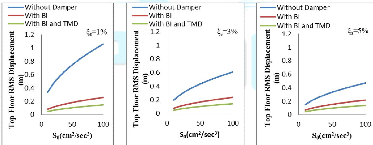
Fig.6 Variation of RMS Displacement of top floor of primary structure with earthquake load for different damping ratio of structure,  $\xi_s$
