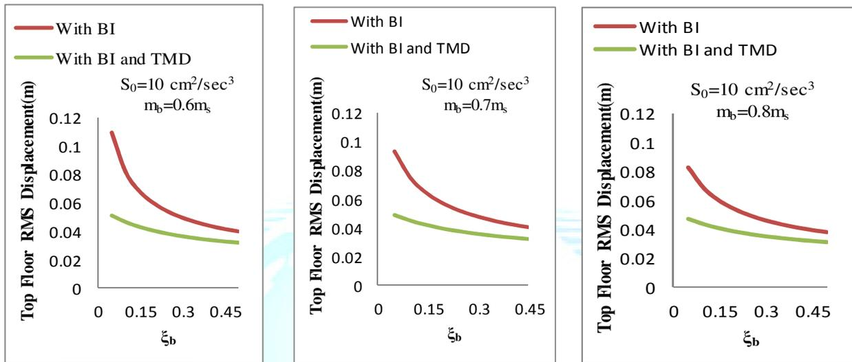
Fig.7 Variation of RMS displacement of top floor with damping ratio of base isolator,  $\xi_b$  for different mass ratio of base isolator and 1% damping ratio of structure,  $\xi_s$  and earthquake load,  $S_0 = 10 \text{ cm}^2 / \text{sec}^3$
