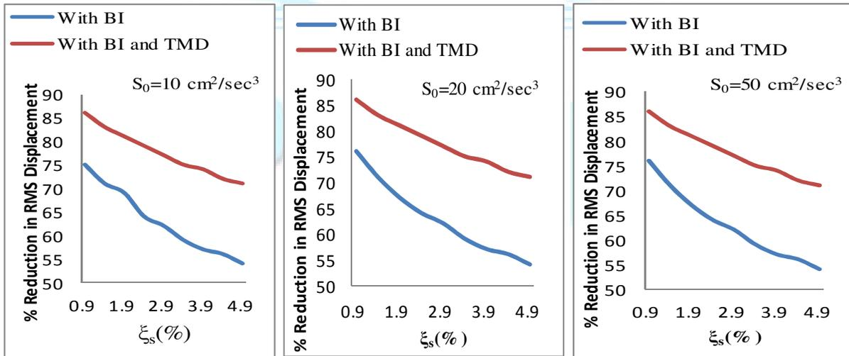
Fig.10 Variation of percentage reduction in RMS displacement with damping ratio of structure for different earthquake load
