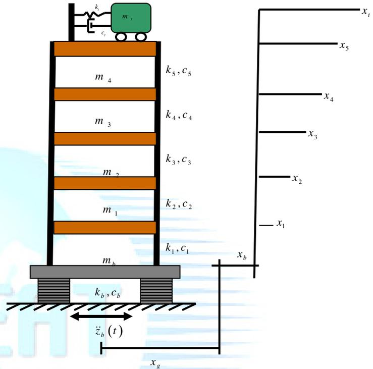
Fig.2 Base isolated structure with TMD
