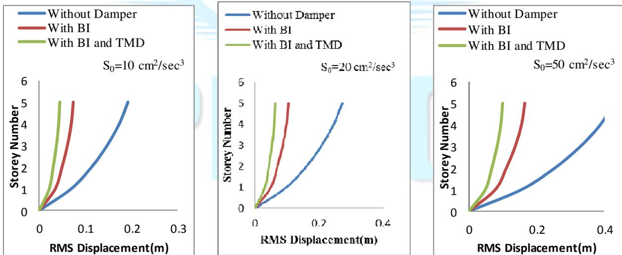
Fig.4 Variation of RMS Displacement of structure with number of story for different earthquake load,  $S_0$  ( $\text{cm}^2 / \text{sec}^3$ ) and damping ratio of structure  $\xi_s = 3\%$
