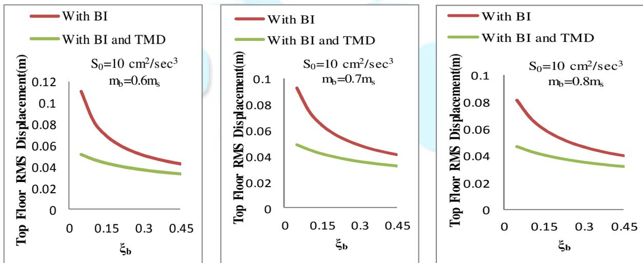
Fig.8 Variation of RMS displacement of top floor with damping ratio of base isolator,  $\xi_b$  for different mass ratio of base isolator and 3% damping ratio of structure,  $\xi_s$  and earthquake load,  $S_0 = 10 \text{ cm}^2 / \text{sec}^3$
