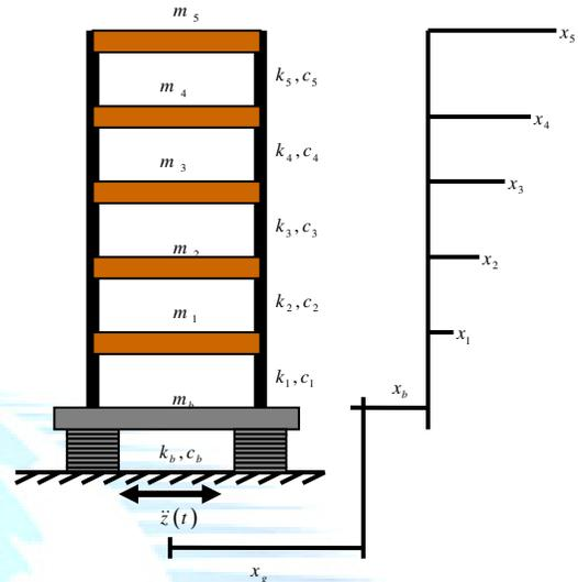
Fig.1 Base isolated structure
