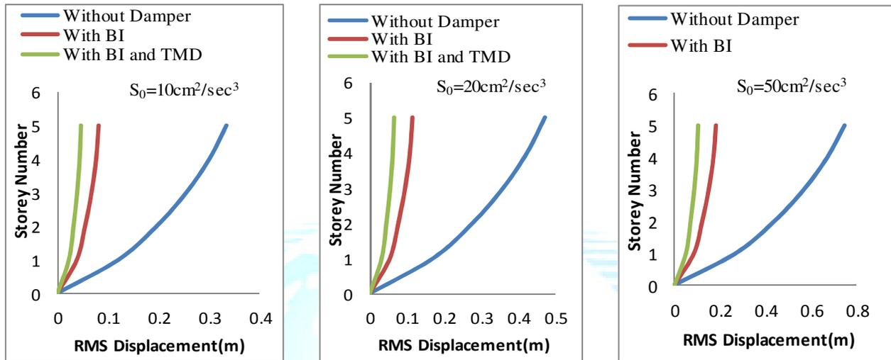
Fig.3 Variation of RMS Displacement of structure with number of stories for different earthquake load,  $S_0$  ( $\text{cm}^2 / \text{sec}^3$ ) and damping ratio of structure  $\xi_s = 1\%$
