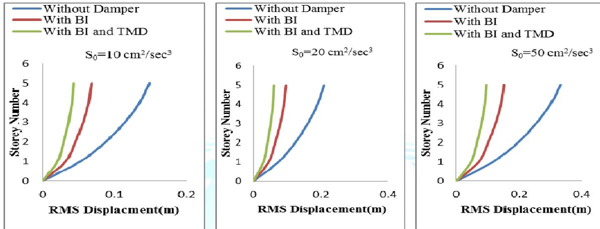
Fig.5 Variation of RMS Displacement of structure with number of storeys for 5% damping ratio of structure and different values of  $S_0$  ( $\text{cm}^2/\text{sec}^3$ )
